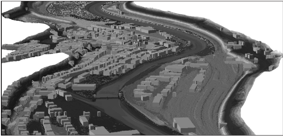
Fig. 15. Correction of a digital terrain model based on laser scanning data [7]
