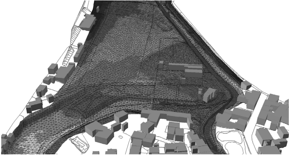
Fig. 10. Mesh structure of the two-dimensional model for the river Kimau in Adelsheim [5]
